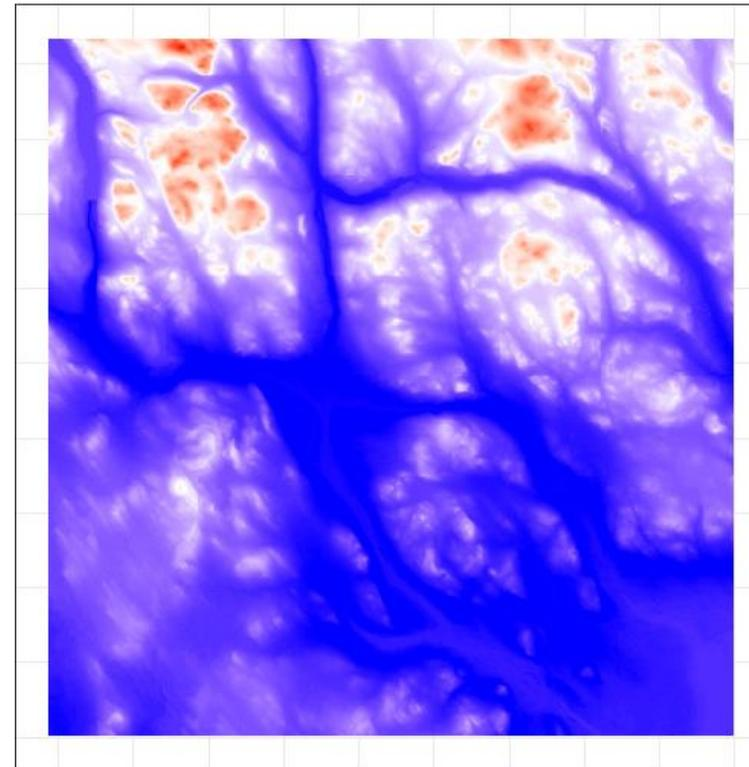
*The ice-loss model produce time series of ice-loss at each turbine. The model also generates an ice-loss map, which enables wind turbine layouts to include the effect of ice-loss already at the planning/optimization stage.*
