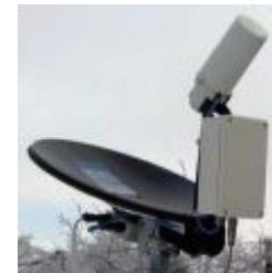
Micro Rain Radar (MRR)
